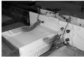
FIGURE 3.7. FOUR BOLT EXTENDED UNSTIFFENED CONNECTION AFTER TESTING (4E-1.25-1.5-24)
