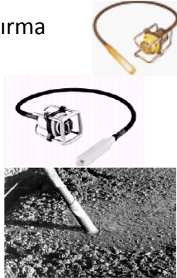
Fig. 4. Internal vibrator: "spigoting" (top) and "needle" (bottom)
